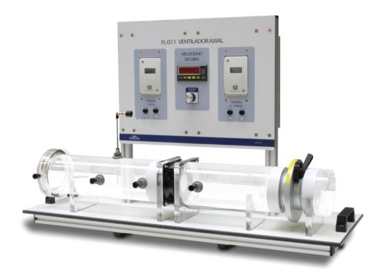
This equipment has been developed for the study of the characteristics of an axial fan, performing a range of experiments and experiences.
